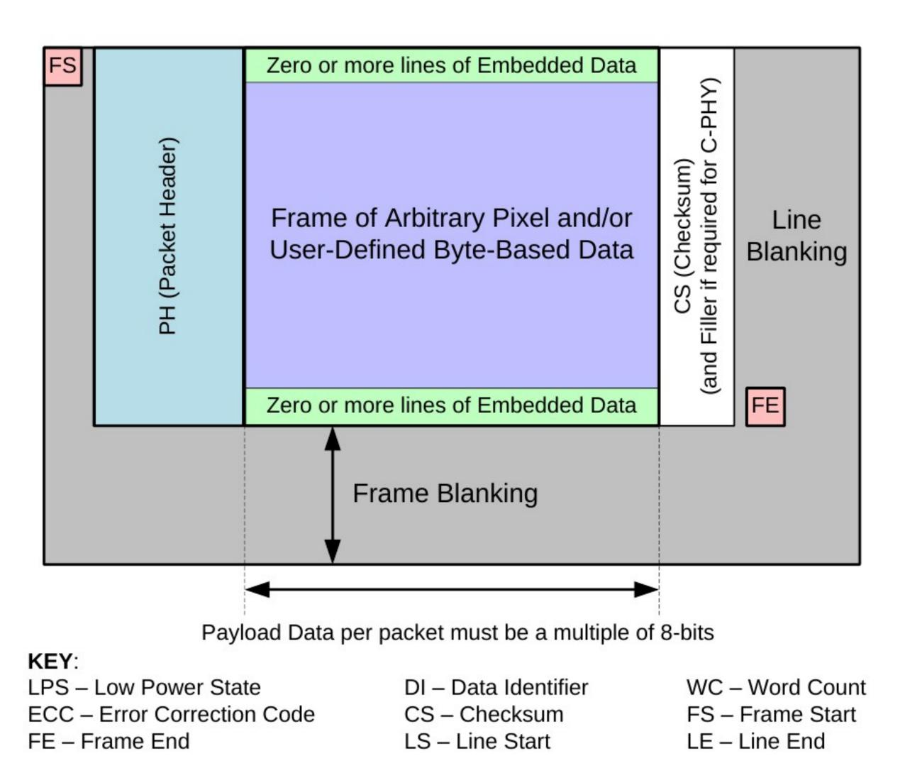
Figure 110 Frame Structure with Embedded Data at the Beginning and End of the Frame
