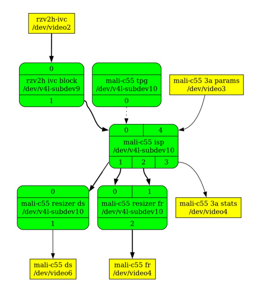
ISP parameters passed through buffers queued on a metadata video device.
